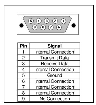
Figure 8 - RS232 Female DCE pin-out
